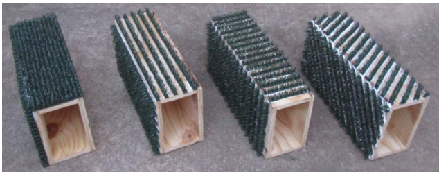
Figure 2. Photographs of the various barrier designs (l to r): control barrier, perpendicular pattern barrier, parallel pattern barrier, and diagonal pattern barrier.
